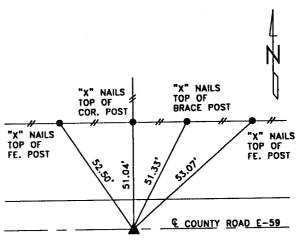
DISTANCES SLOPE CHAINED SE CORNER SECTION 9-82-39
