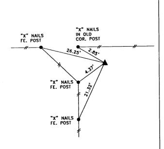
DISTANCES SLOPE CHAINED E1/4 CORNER SECTION 9-82-39
