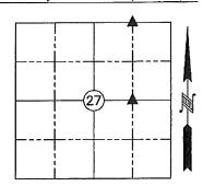
NW CORNER NE1/4 NE1/4 SEC. 27, T82N, R39W (Set a 5/8" dia. rebar w/orange cap PLS #17048, 0.6' deep)
