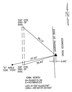
DISTANCES PLUMB CHAINED NE CORNER NW1/4 NW1/4 SECTION 10-82-40
