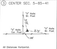
SET 5/8" DIA. BY 24" REBAR W/ORANGE CAP PLS #17048 — FLUSH.
