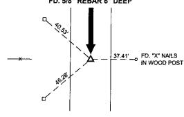
□ = 5/8" REBAR WITH ALUM, CAP STAMPED "SECTION CORNER REF. PT.
