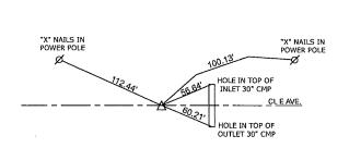
ALL TIE DISTANCES ARE MEASURED HORIZONTALLY USING GPS
