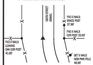
NO RECORDED TIES FOUND. USED COUNTY ENGINEER'S TIES TO FIND 5/8" REBAR WITH YPC 8893 4" DEEP. MANY OF THE TIES ARE STILL THERE AND FIT WELL. ACCEPTED MONUMENT AND RETIED SINCE THERE ARE NO CURRENT RECORDED TIES.
