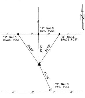
DISTANCES SLOPE CHAINED S1/4 CORNER SECTION 31-82-38
