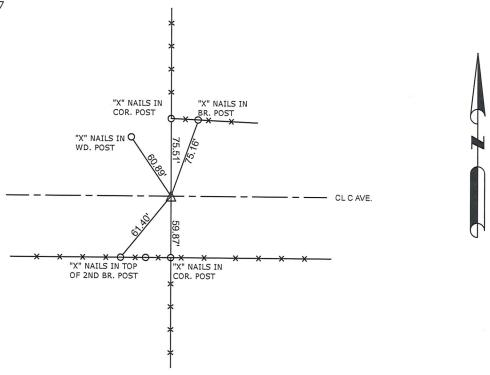
ALL TIE DISTANCES ARE MEASURED HORIZONTALLY USING GPS
