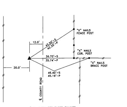
46.40'-S DISTANCES SLOPE CHAINED 45.19'-P DISTANCES PLUMB CHAINED E1/4 CORNER SECTION 36-84-40
