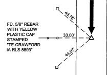
□ = 5/8" REBAR WITH ALUM. CAP STAMPED "SECTION CORNER REF. PT.
