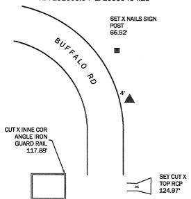
TIES FROM FEE BOOK 2007-1626 HAVE BEEN TORN OUT FROM THE RECONSTRUCTION OF BUFFALO ROAD IN THIS AREA. COUNTY SURVEYOR STILL HAD POINTS IN HIS DATA COLLECTOR AND LOCATED THIS POSITION. DUG DOWN 1.5' AND FOUND A SHORT 5/8" REBAR. RESET POSTION WITH 24"x5/8" REBAR 4" DEEP.
