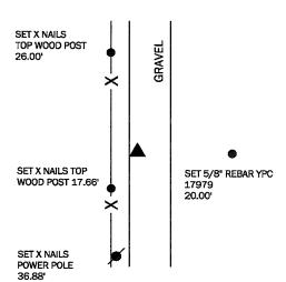
USED TIES RECORDED IN FEE BK 2007-1624 TO START SEARCH. TIE MONUMENTS DID NOT HAVE CROSS NAILS AND WAS A LITTLE UNSURE OF POSTION. DUG 1.5' AND FOUND BRICKS & JUNK. COUNTY SURVEYOR STILL HAD POINTS IN DATA COLLECTOR FROM A PAVING JOB TO THE EAST AND STAKED OUT THE POSITION. DUG TO A DEPTH OF 2.7' AND FOUND 5/8" REBAR. FILLED HOLE AND SET 5/8" REBAR WITH YPC 17979 3" DEEP.
