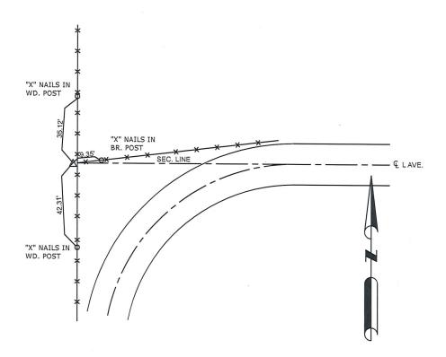
ALL TIE DISTANCES ARE MEASURED HORIZONTALLY USING GPS
