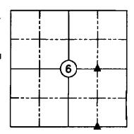
NE CORNER NW1/4 SE1/4 SEC. 6,783N, R38W (Set 5/8" dia. by 24" rebor w/orange cop PLS \$17048, flush with ground)
